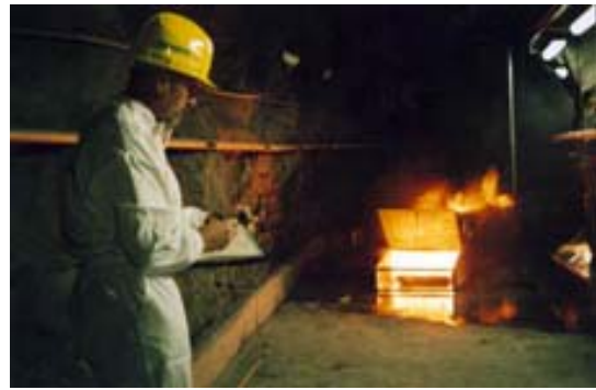
The test with dummy vehicle and a tunnel wind of ~ 5m/s at fire source
