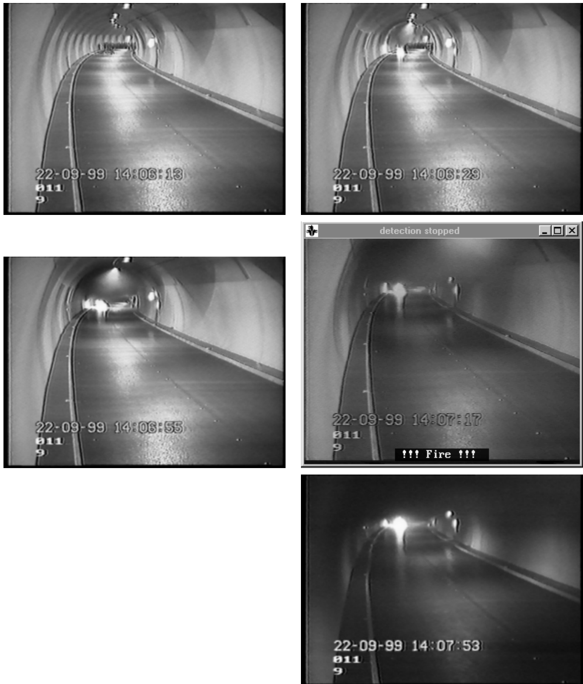
Figure 3: Screen shots of the large scale test in the Schönberg tunnel near Salzburg. Width of tunnel = 10 m, height = 6 m. Wind speed 1.0 – 1.2 m/s. Area of fire 1 m 2 , 20 L gasoline with 5 L diesel added. Distance between camera and fire 60 m
