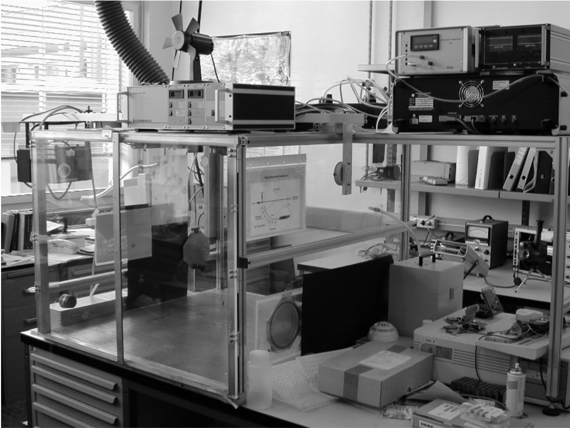
Figure 2: The smoke box used to develop and calibrate the algorithm.
