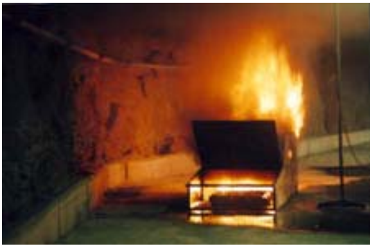
The test with dummy vehicle without tunnel wind at fire source
