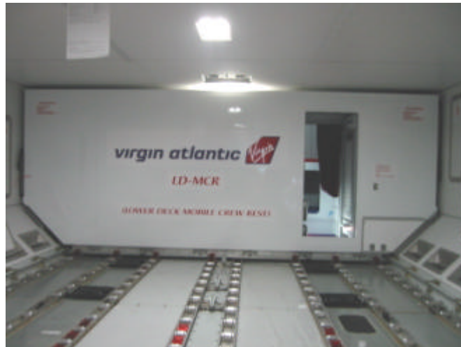
Fig. 4: Lower Deck Mobile Crew Rest Compartment
