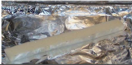
Soft polyurethane foam without flame retardant additives. Size: 4x2 x40cm 3 , (20kg m -3 )
