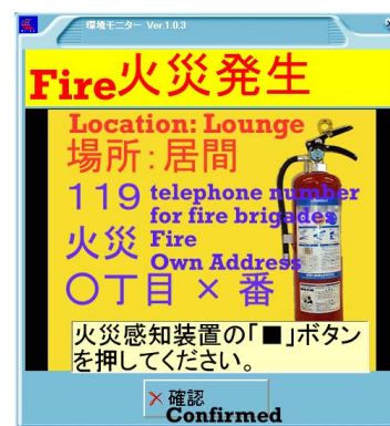
Fig. 6b: Fire alarm displayed on the TV screen
