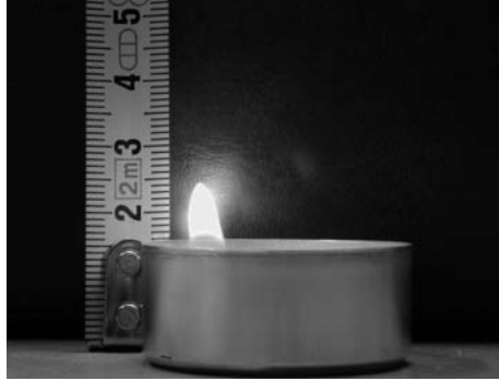
Figure 1: Greyscale image of the candle used as a source for flame detection
